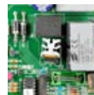
D24 Control board for Daphne barriers.
